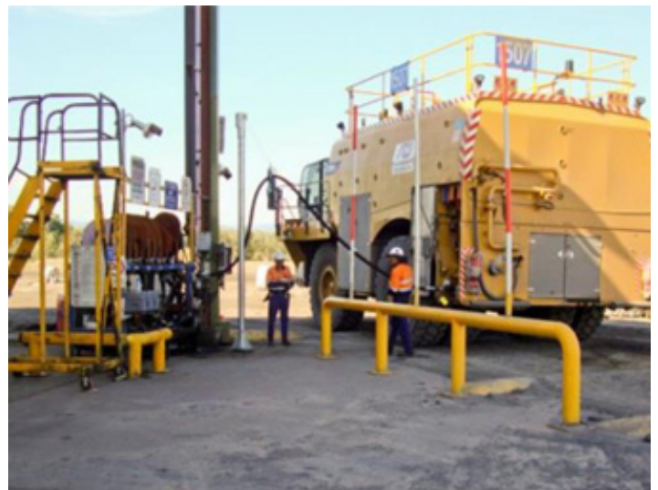
Figure 1 – Counter-weight Dispensing Tower In Use
